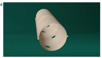
The bottom sheet contains holes, allowing air to be discharged onto calves once the duct is inflated.
