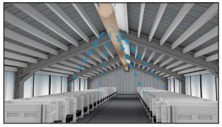
Many of these systems use low-output fans connected to small diameter ducts to deliver low volume, slow air for winter ventilation. They work well for winter. But they lack the ventilation power needed for warmer weather conditions.
