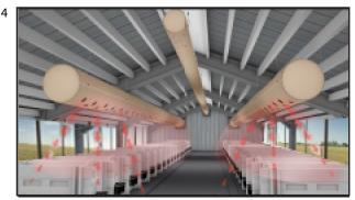
Some farms are now adding high-output fans connected to large ducts to deliver more ventilation power during warm weather. These systems work well, yet require more fans, ducts, controllers, and electricity – resulting in increased costs for a system used only 3 to 4 months each year.
