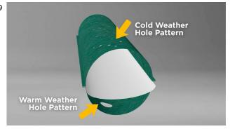
FLIP DUCT® is manufactured with a patent-pending internal liner membrane sewn into the middle of the duct. The liner allows a cold weather hole pattern to be placed on one side of the duct and a warm weather hole pattern on the opposite side.
