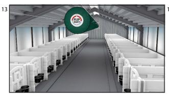
Metal snaps securely sewn into the sides of FLIP DUCT® attach to the cables at 3 and at 9 o'clock. Vertical cables suspended from the barn roof attach to the horizontal cables, preventing sag.
