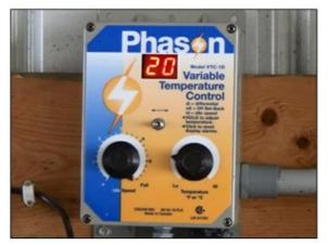
**Phason VTC-1D**How to set the Phason VTC-1D variable speed controller.
