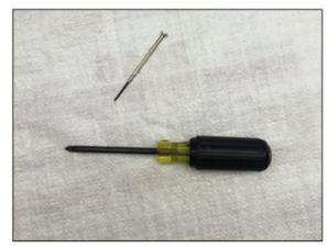
**Tools needed**A medium sized Phillips screwdriver and small flathead screwdriver are needed to set the controller.
