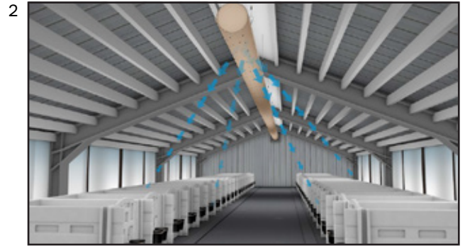
Many of these systems use low-output fans connected to small diameter ducts to deliver low volume, slow air for winter ventilation. They work well for winter but lack the ventilation power needed for warmer weather conditions.
