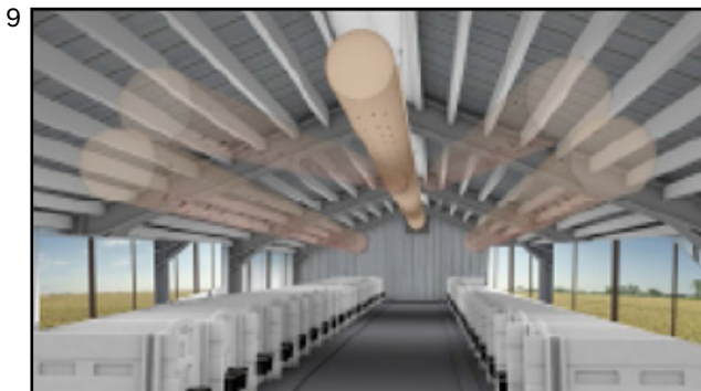
This single-duct system combines a cold-weather duct with a warm-weather duct, providing proper calf barn ventilation all year round.
