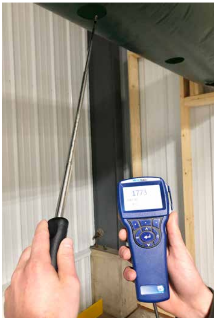
Picture 1: A hot wire style air speed meter is used to measure air speed and volume from a positive pressure tube.
