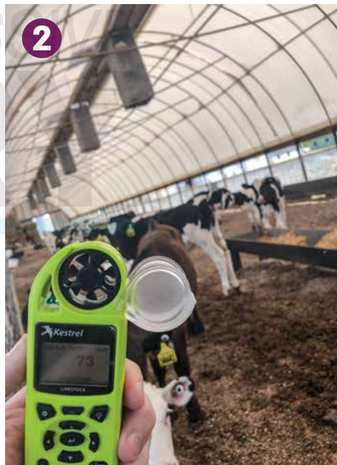
A windmill-style air speed meter is used to measure air speed.
