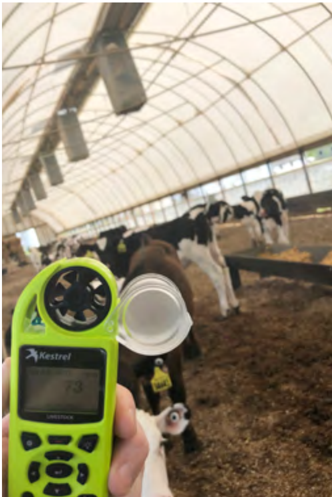
Picture 2: A windmill style air speed meter is used to measure air speed.
