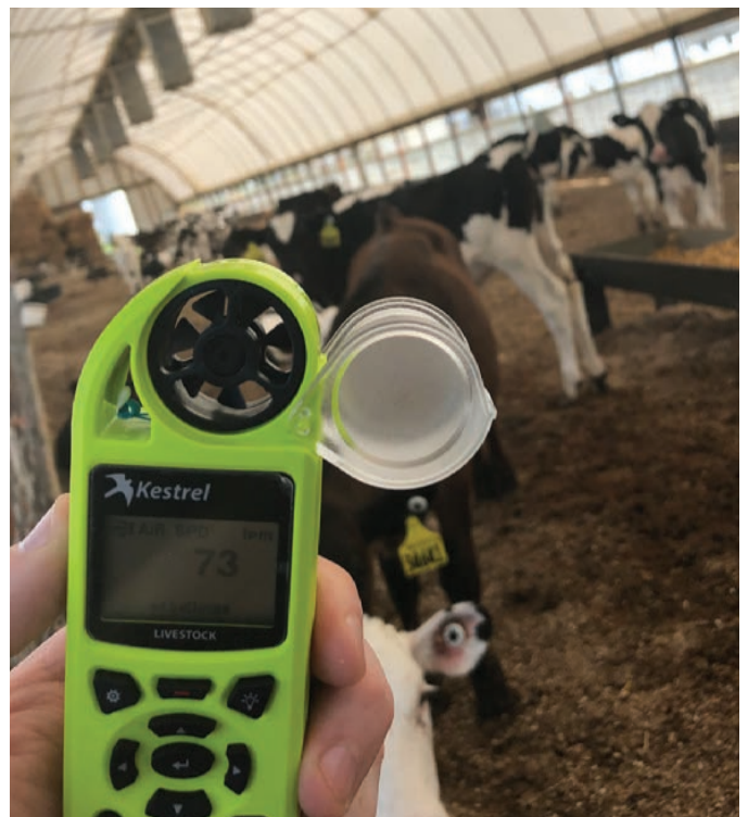
An anemometer is a windmill-style air speed meter.
