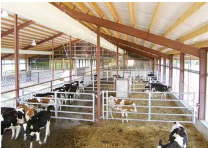
Picture 2: These 18 inch knee walls create better airflow at the level of the calves.
